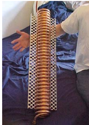
Figure 6 Heat exchanger midway through fabrication. The copper coils thread into the holes that were water jetted into the stainless steel plate.
